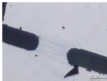
Fig. 1 optical image of circular electrodes( $\rho=30 \mu\text{m}$ )
