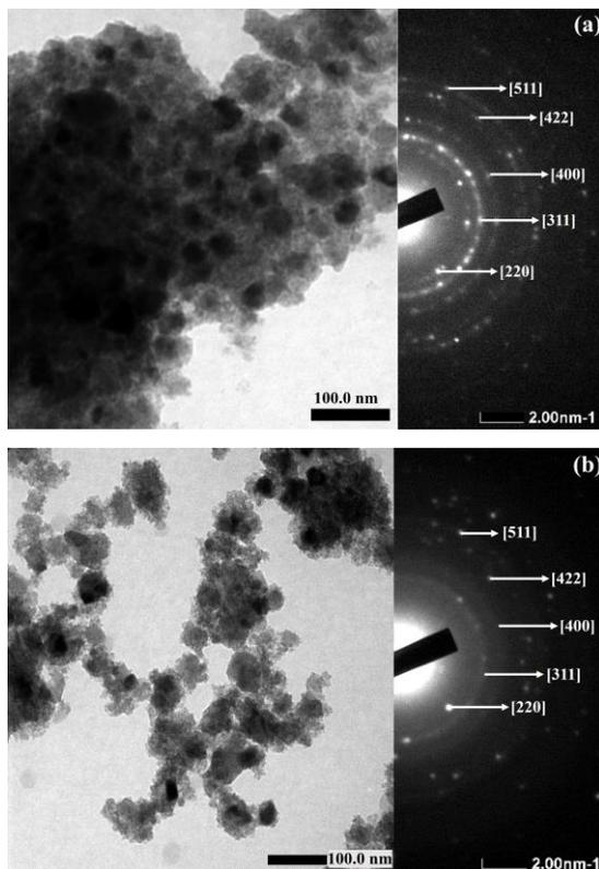
Fig. 3. TEM images of  $\text{CoZnFe}_2\text{O}_4$ : (a) as prepared, (b) Encapsulated by silica 50%.
