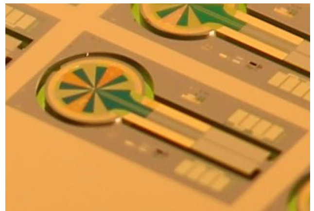
Fig. 1 An image of microcalorimeter devices composed of TES and optical cavities on a Si substrate cut by deep RIE.
