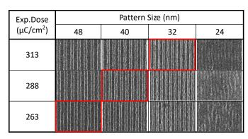
Fig. 1 SEM images of low molecular weight compound-based resist material patterned using EB lithography.
