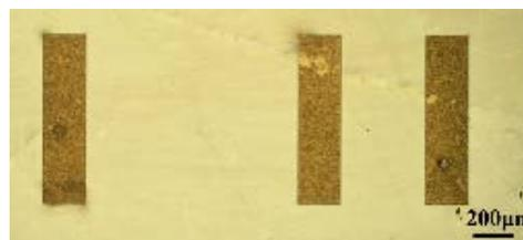
Fig. 1 Pictures of ohmic electrode after annealing
