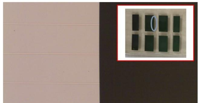
Fig. 2 Optical image of SOI after cleavage.
