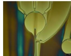
Fig. 1 CCD image of a silicon mold fabricated by dry etching.
