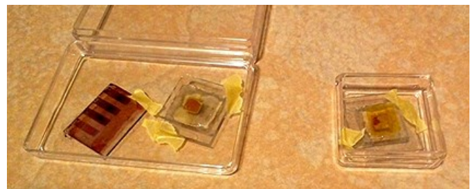
Fig. 1 Organic thin-film (Left) and dye-sensitized solar cells.
