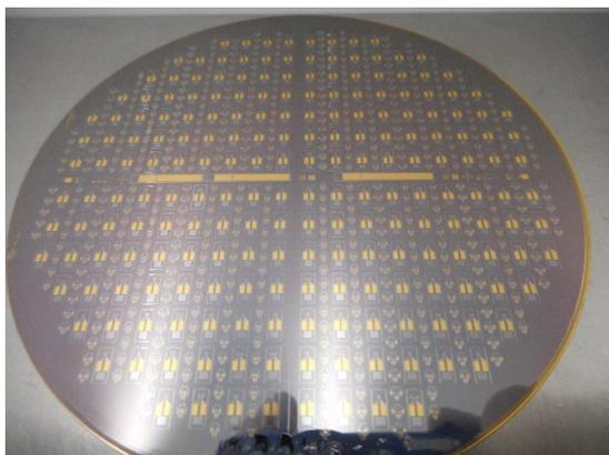
Fig. 1 Photograph of dry-etched Si wafer.
