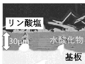
Fig.2 Cross-sectional SEM image of hydrothermally treated Mg alloy.
