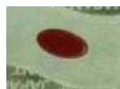
Fig4. Picture of the surface on the red ink after the deposition of Al 2 O 3
