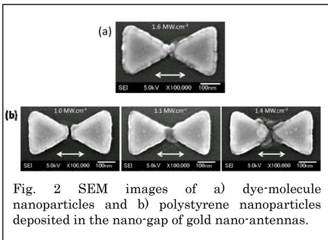
Fig. 2 SEM images of a) dye-molecule nanoparticles and b) polystyrene nanoparticles deposited in the nano-gap of gold nano-antennas.
