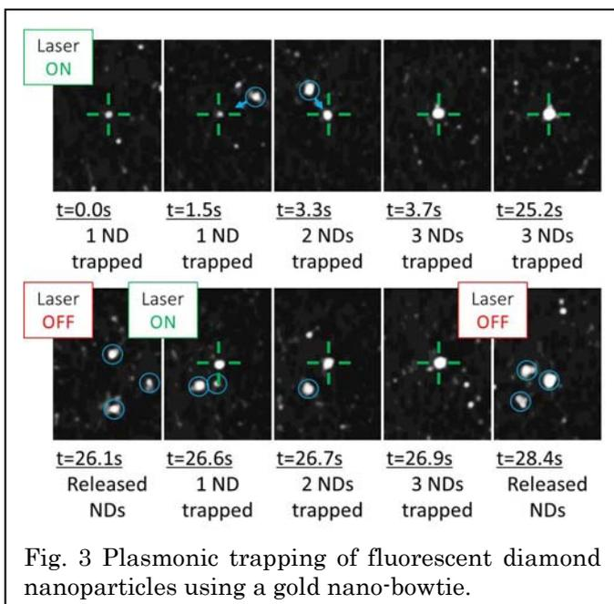
Fig. 3 Plasmonic trapping of fluorescent diamond nanoparticles using a gold nano-bowtie.
