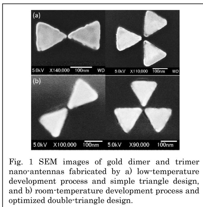
Fig. 1 SEM images of gold dimer and trimer nano-antennas fabricated by a) low-temperature development process and simple triangle design, and b) room-temperature development process and optimized double-triangle design.
