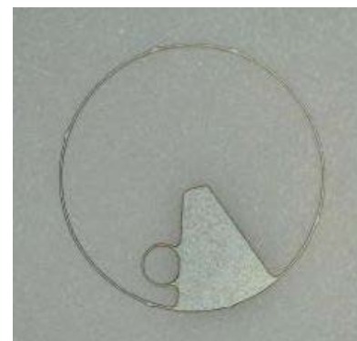
Fig. 2 SUS ring to which the fabricated micromirror is bonded.
