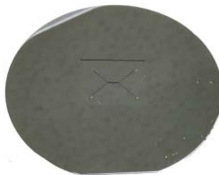
Fig. 1 Picture of molding template for microfluidic devices fabricated on 4-inch silicon wafer
