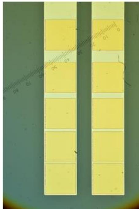
Figure 1 Picture of metal electrode pattern.
