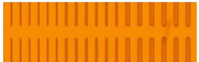
Fig. 1 OM image of photoresist on SiO 2 /GaN surface.
