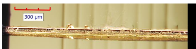
Fig. 1 Overview of waveguides after dicing with angled blade.
