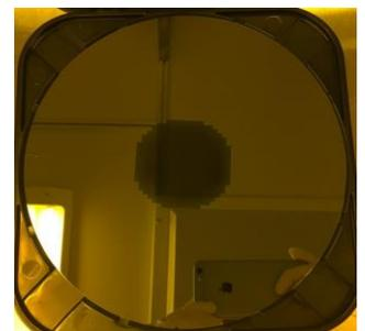
Fig. 1 Photo of Si mold.
