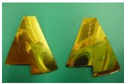
Fig.1 Upper- and lower-electrodes after Au deposited.
