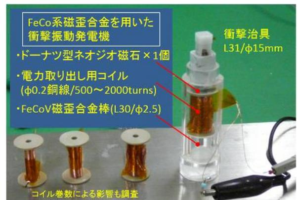
Fig. 1 A prototype of impact vibration power generator studied in this work.
