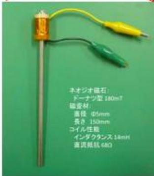
Fig. 3 Outer view of the actuator produced in this work.
