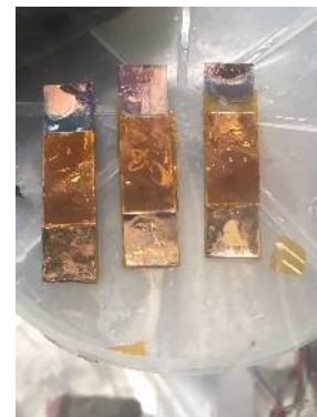
Fig.1 Photograph of Si-O-C composite anode (electrodeposition on an evaporator substrate).
