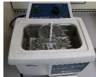
Fig.2 Cleaning by an ultrasonic cleaning device.
