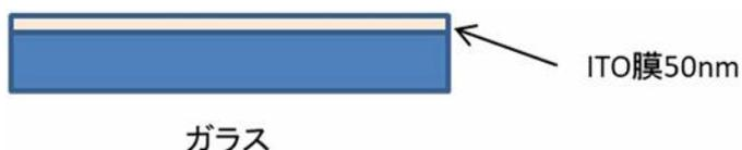
Fig.1 Substrate for plating
