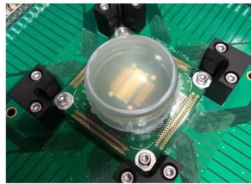
Fig. 2 A fabricated multi-channel ultrasound transducer in this work.
