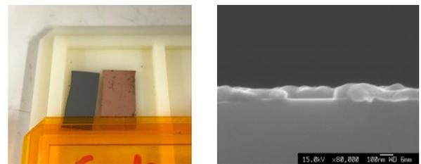
Fig. 1 (Left) Si substrate before and after Cu-SCFD. (Right) Cross-sectional SEM image of the Cu-deposited sample.
