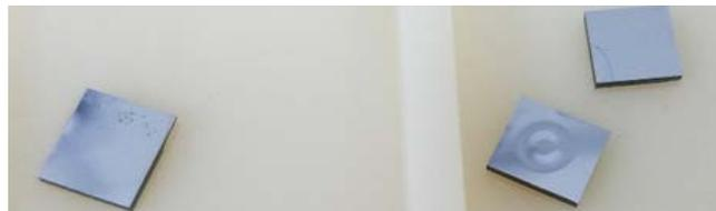
Fig. 3 Fabricated MEMS Pressure sensor chips
