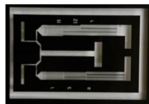
Fig. 1 Chromium mask made by EB
