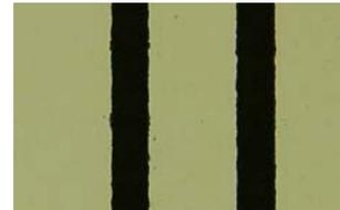
Fig. 2 Optical microscope image of slit pattern in silicon stencil mask.
