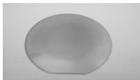
Fig. 1 Picture of PZT thin-film fabricated by Sol-gel method on Pt/SiO 2 /Si wafer.
