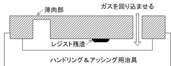
Fig .3 Special tool for chip handling
