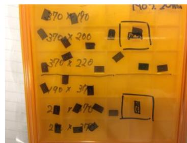
Fig. 2 The chips diced from the Si wafers.
