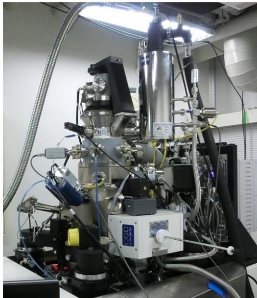
Fig. 1 high definition focused ion beam system ZEISS “ORION NanoFab”
