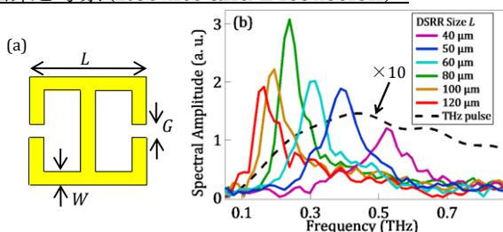
Figure 1(a). Dimensions of double split ring resonator. (b) The spectra of the enhanced THz magnetic near-field.
