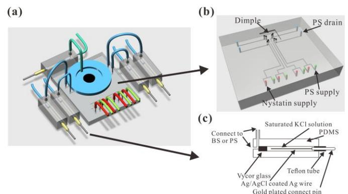
Fig. 2. (a) Schematic figure of the incubation-type planar patch clamp device used in this work. (b) 3D image of the microfluidic plate. (c) Illustration of the salt-bridge stable electrode. PS: pipette solution; BS: bath solution.
