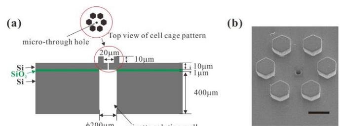
Fig. 1. (a) Schematic cross section image of the planar patch clamp chip fabricated by Bosch process. (b) SEM image of the chip surface with micro-through hole and cage structure. Incident angle is 15 degrees. Scale bar is 10 μm.
