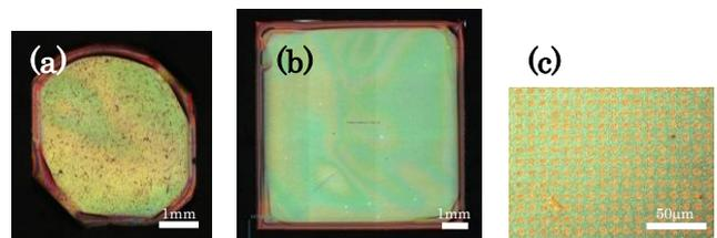
Fig. 1 Optical microscope images after photolithography. (a) HPHT (b) CVD (c) Resist pattern
