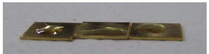
Fig. 1 Digital Photograph of the aqueous droplet on the prepared thin films of the electrode materials. (Left) As prepared, (Center) Hydrothermally treated in alkaline aqueous solution, (Right) Carbon coated and subsequently hydrothermally treated in alkaline aqueous solution.
