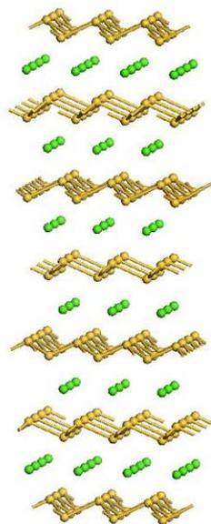
Fig.1 Crystal structure of  $\text{CaSi}_2$ .
