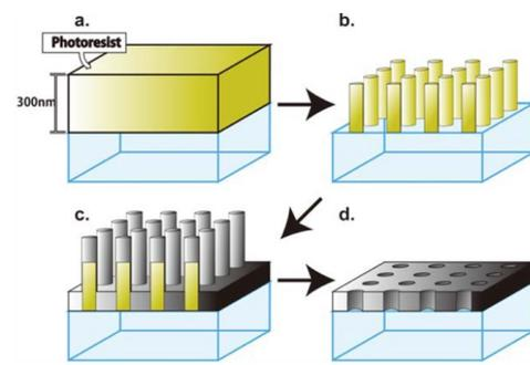
Fig. 1 Schematic diagram of Zero Mode Waveguides fabrication. (a) Photo resist coating. (b) Fabrication of the resist pattern by electron beam lithography. (c) Vapor deposition of aluminum. (d) Removal of the resist film.
