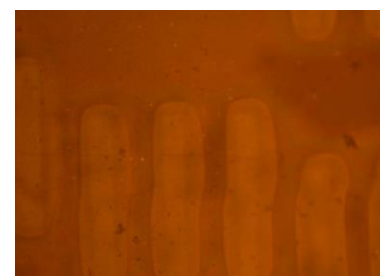
Fig. 1 Patterning result of EB exposure (500 \mu\text{C}/\text{cm}^2 ) #1
