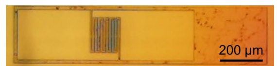
Fig. 2 An optical microscope image of a device pattern on a diamond substrate.
