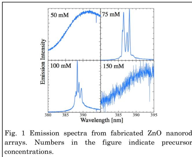
Fig. 1 Emission spectra from fabricated ZnO nanorod arrays. Numbers in the figure indicate precursor concentrations.
