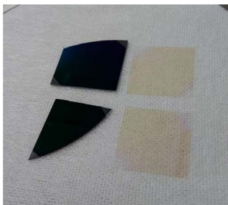
Fig.1 Deposition on glass substrate and silicon substrate
