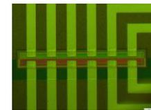
Fig. 2 Microphotograph showing the strain sensor with interconnect metallization.
