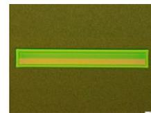
Fig. 1 Microphotograph showing a Si sensor island implanted with P and  $\text{BF}_2$  ions.
