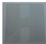
Fig. 1 Photograph of the ITO thin film heater.
