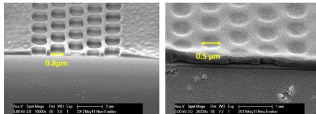
Fig. 1 SEM images of (a) 0.8  $\mu\text{m}$   $\phi$ , (b) 0.5  $\mu\text{m}$   $\phi$  hole patterns.
