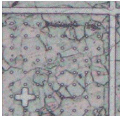
Fig. 1 Optical image of the artificial pits fabricated on the SUS304 plate.
