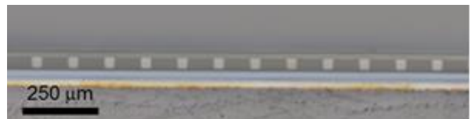
Fig. 1 A cross-section of polymer optical waveguide.
