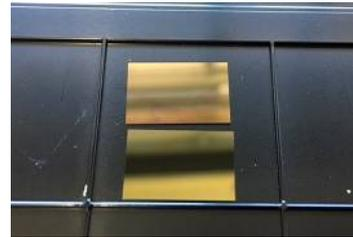
Fig. 1 Appearance of Si wafer after wet oxidation process.
