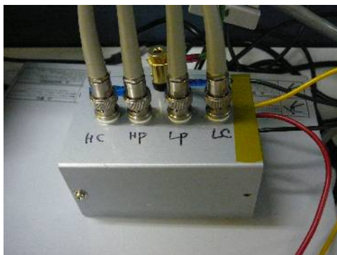
Fig. 1 Photograph of a conversion connector.
